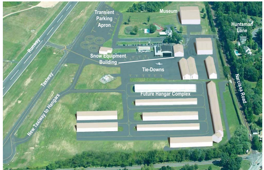
This aerial view depicts how Wings Field might appear in the future after the infrastructure improvement projects envisioned by the airport are completed. The plan envisions an increase in the number of aircraft stored in locked hangars, a proportional decrease in the number stored in outside tie-down spaces, with no significant change in the overall capacity of the airport.
