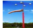
Landings and takeoffs are always made into the wind. Pilots, therefore, need a visual cue to indicate wind direction. Wind socks are made of flexible fabric and pivot freely to point downwind and show the direction of the wind. Pilots estimate wind velocity by noting whether the sock hangs limply or is stretched straight out. The Wings wind sock is located alongside the runway.
